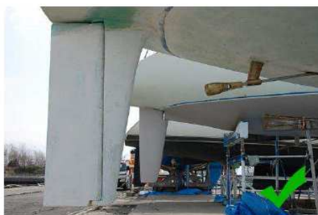
Skeg clearly visible as is propeller
